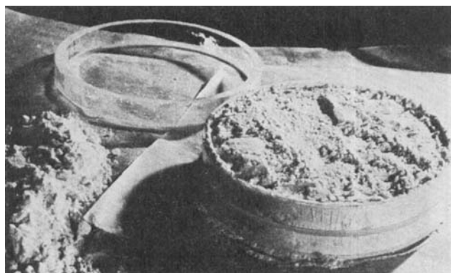
Figure 3 —Drying cell used in the study of drug migration shown after the top ring has been sampled and removed. The second level is now exposed and ready to be sampled.
